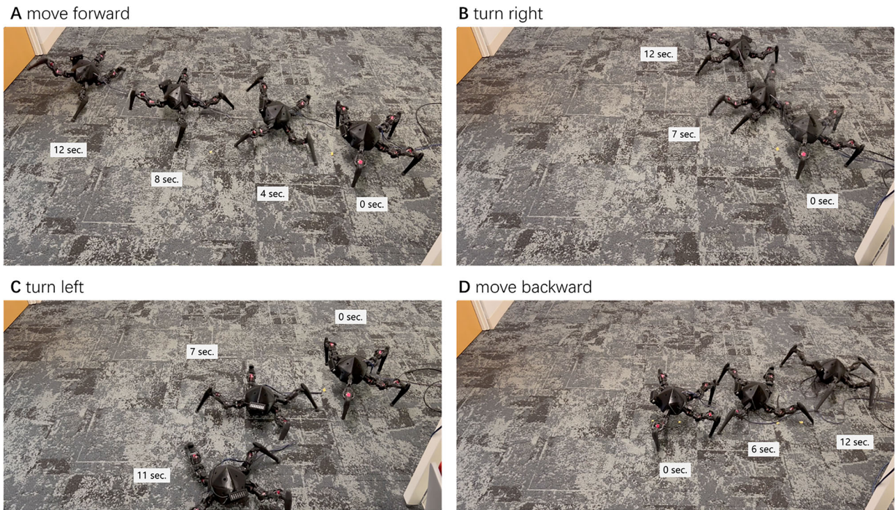
Fig. 2 | Basic locomotion tasks in the real-world environment. We deployed an egocentric visual self-model on a legged robot. The robot only relies on image sequences from the front camera and action commands to achieve (A) moving forward, (B) turning right, (C) turning left, and even (D) moving backward. It learns
